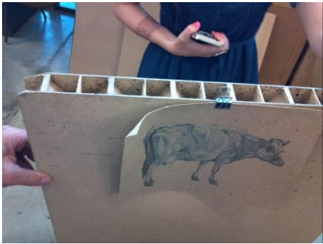
Panel from recycled cardboard and cow manure Uses: hollow-core doors, modular furniture, theater stage sets
