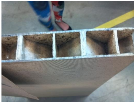
Panel from recycled cardboard and cow manure Uses: hollow-core doors, modular furniture, theater stage sets
