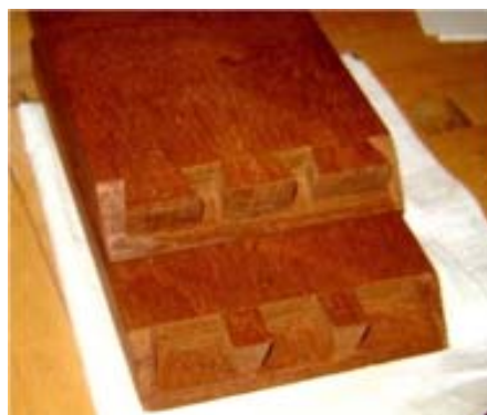
Making Handcut Dovetails
